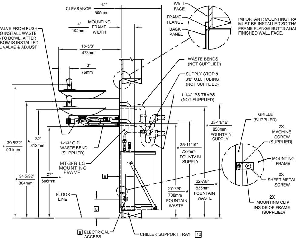
IMPORTANT: MOUNTING FRAME MUST BE INSTALLED SO THAT FRAME FLANGE BUTTS AGAINST FINISHED WALL FACE.
